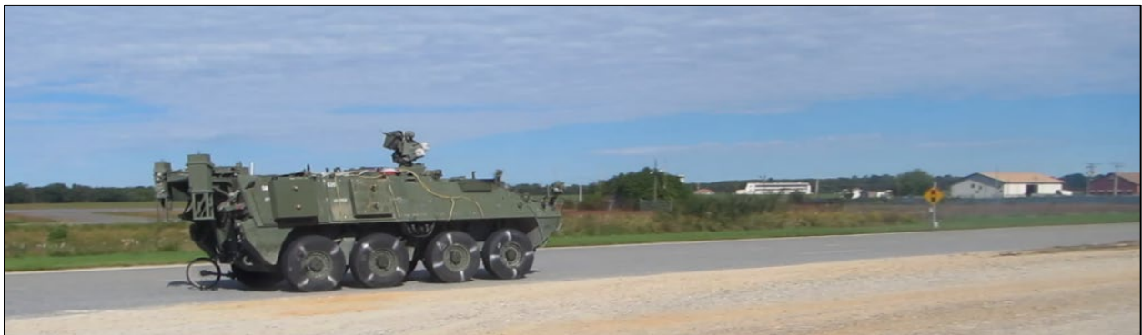
Photo Source: Aberdeen Test Center: The Stryker DVH A0 on the ATC test track during spherical brake FMVSS121.
